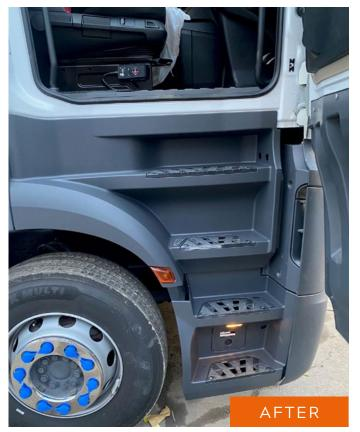
**3. Final Touches:** After completing the repairs, the vehicle was primed and painted, ensuring that the vehicle was aesthetically pleasing and ready for use.
