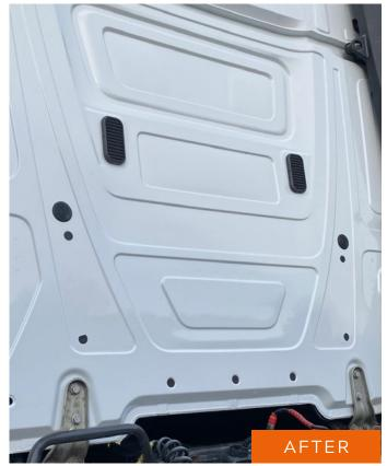
**2. Panel Repair:** After the bulkhead repair, we proceeded to complete extensive panel repairs across the vehicle, including re-texturing to ensure the panels matched the vehicle's original finish.
